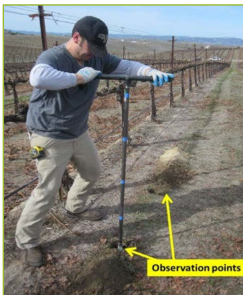
Figure 4: Before installing soil moisture sensors under the drip line, a series of observation points can be evaluated at a short distance from the desired sensor placement location. This extra step can verify that the soil is representative and identify abnormalities in soil that can influence water movements, such as hard pans, or pockets of rock or sand.
