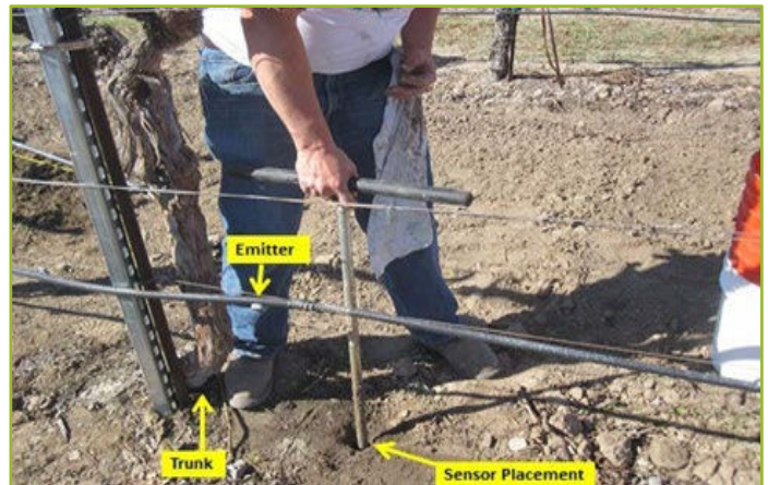
Figure 2: A typical soil moisture sensor installation showing the placement distance no more than 18 inches from the vine trunk, and 4-6 inches from a drip emitter.
