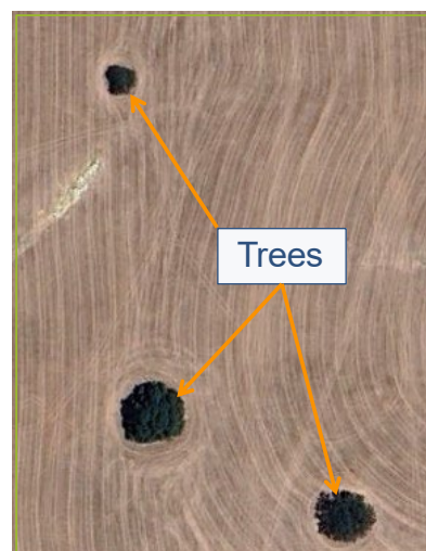
Figure 5: Trees or other objects that may disturb soil during the removal process should be mapped and those areas avoided when installing soil moisture sensors. Sensors installed in disturbed areas such as these may not be representative of conditions in adjacent undisturbed areas.
